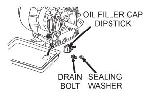
Figure 16. Engine Oil Plug
